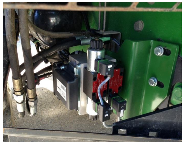
FIGURE 4 MOUNTED MANIFOLD AND HYDRAULIC DRIVE UNIT
