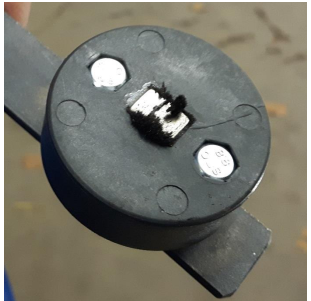
FIGURE 26 DIRTY WHEEL ANGLE SENSOR MAGNET
