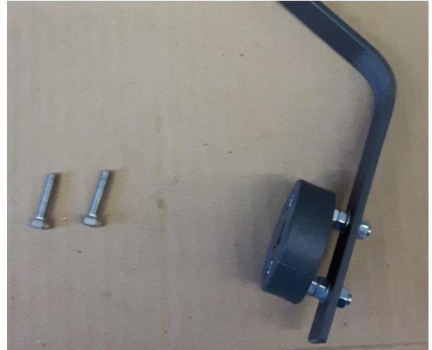
FIGURE 25 WHEEL ANGLE SENSOR DISC MOUNTED WITH SPACERS
